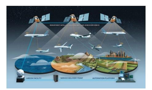
ADS-B information broadcast from aircraft will be received by Aireon's ADS-B hosted payloads on the Iridium NEXT satellite constellation. It is then relayed to air traffic control facilities in real time.
